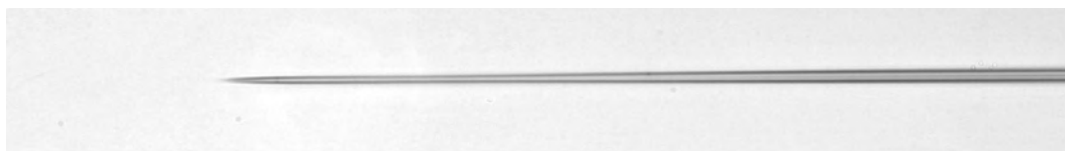
0.7 - 0.9 \mu m tip, 5 - 7mm taper (400x)
