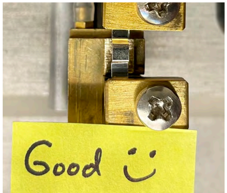
Box filament is centered over the air jet (GOOD)
