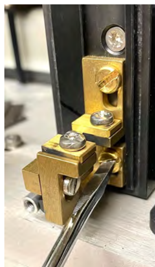
STEP 3. Loosen bottom brass screw.
