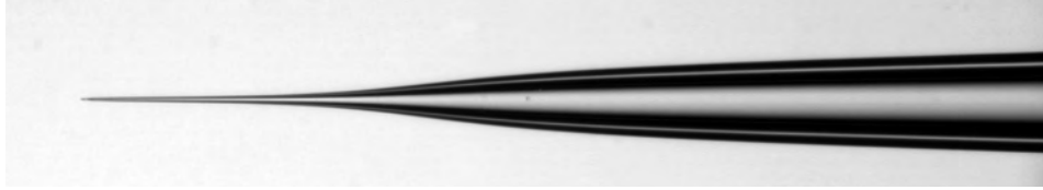
Image A (40x mag.) 1.0 x 0.5 thick-walled glass (BF100-50-10) ~0.5 \mu m Tip, 4-5mm taper, one line program with 3 loops
