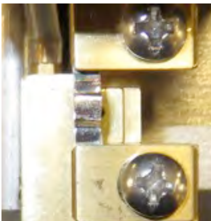
Box filament is not centered over air jet (BAD)
