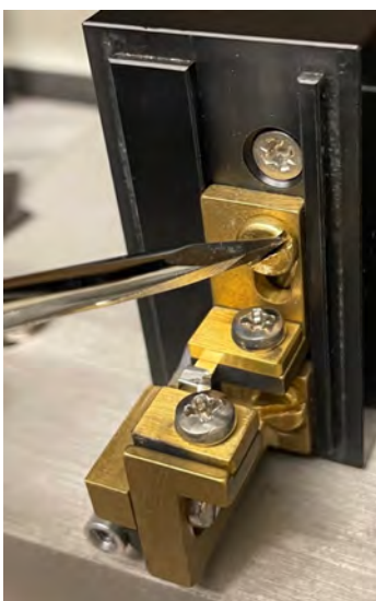
STEP 1. Loosen top brass screw.
