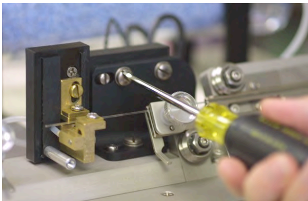
Loosen the locking screw
