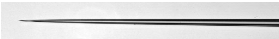
0.6 - 0.9 \mu m tip, 6 - 8mm taper (400x)
