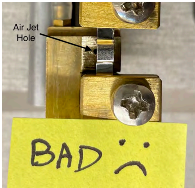
Box filament is not centered over air jet (BAD)
