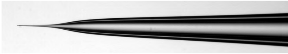
Image B (40x mag.) 1.0 x 0.5 thick-walled glass (BF100-50-10) ~0.5 \mu m Tip, w/ a shorter taper than that shown above. Three-line program with a reduced velocity on Line 3
