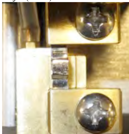
Box filament is not centered over air jet (BAD)
